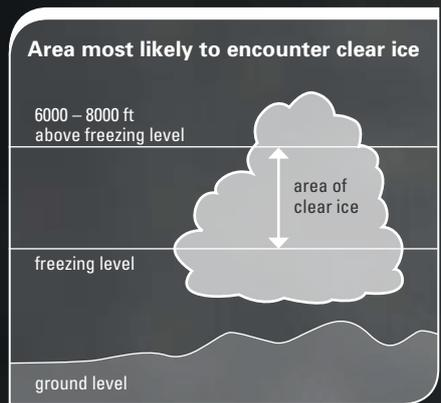
Clear ice is dangerous for many reasons. It can quickly build up – dramatically increasing the aircraft weight and stall speed. It can spread back over a large area and can be difficult to detect, particularly at night. Initially, it may not affect aerodynamic performance, but if allowed to flow back to the hinge line of a control surface, it may render the control unusable. When the aircraft encounters warmer air, it can break off in large chunks, possibly causing airframe damage.
