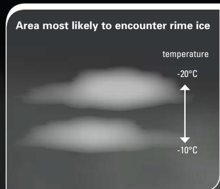
It dramatically affects the aerodynamic qualities of leading edges, but unlike clear ice, it does not usually cause a significant increase in aircraft weight. It can be easily cleared using de-ice equipment.
