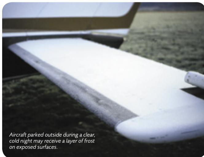
Aircraft parked outside during a clear, cold night may receive a layer of frost on exposed surfaces.
